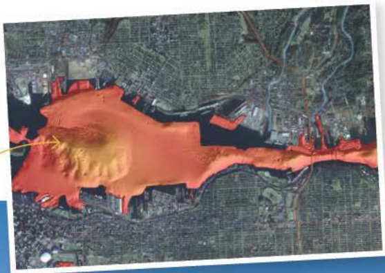
This multi-beam image shows the large, shallow sill at the entrance of Vancouver's busy harbour.
