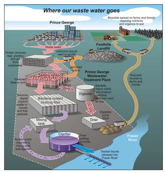
Figure 17. (Left) Waste water arriving at the treatment plant. Solids are trapped and removed on screens.
