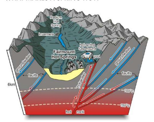
**Figure 91.** The natural geological plumbing system for Fairmont Hot Springs.
