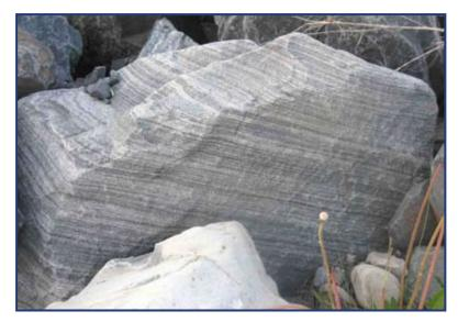
Figure 66. (Left) Sandstone blocks that make up the dykes contain layering and (Right) carbonized plant fragments.
