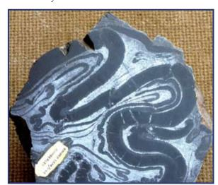
Figure 26. The ores of the Sullivan mine are composed of fine layers of zinc and lead sulphide (silver) and mud (black). Geologists interpret that these layers formed on a sea floor near a submarine hot spring. The layers were originally flat. During mountain building starting 170 million years ago, the layers were deformed into folds.
