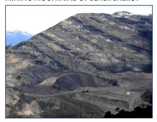
Figure 81. (Left) Tilted layers of grey sandstone and shale and black coal seams are exposed in a wall of the Greenhills coal mine north of Elkford. Horizontal lines are benches cut into the wall. The giant coal truck in the bottom of the mine provides a scale.
