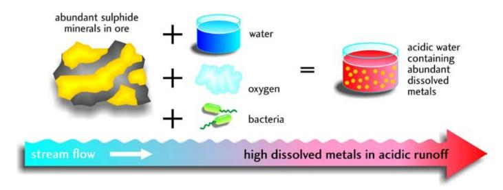
Figure 28. (Left) The formula for the formation of acid rock drainage.
