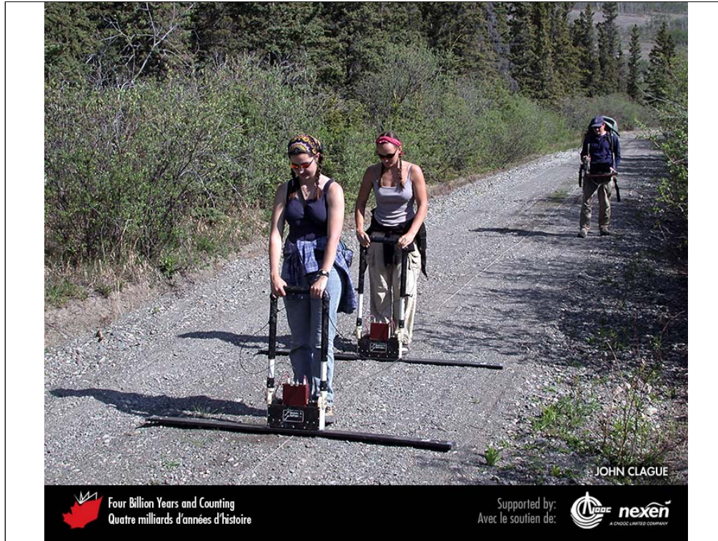
Ground-penetrating radar survey, Kluane Lake, Yukon. JOHN CLAGUE.
